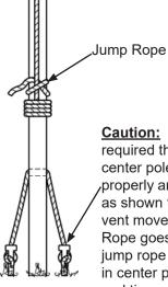
**Caution:** It is required that all center poles be properly anchored as shown to prevent movement. Rope goes thru jump rope hole in center pole and ties around stakes.
