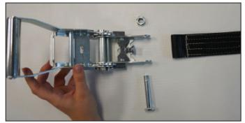
2. Move ratchet to an open position (Reference step one in Release Instructions). Remove nut and bolt.
