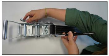
3. Position web loop in line with bolt holes on the ratchet body. Insert bolt through web and fasten with nyloc nut.
