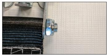
4. Ensure bolt is tightened so that it is at least three thread lengths past the nylon ring on the nyloc nut.
