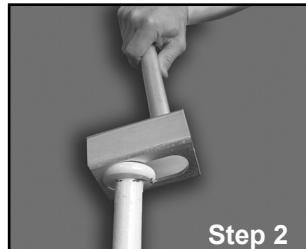
**Step 2:** Fit adapter over head of stake and slide into small end of slot.
