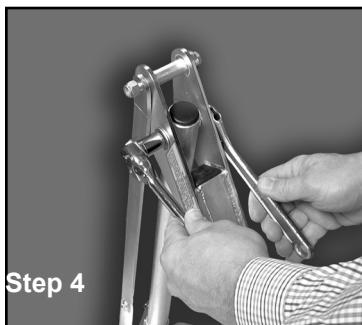
**Step 4:** Use two 9/16" wrenches to tighten riser bolts and nuts and link arms onto handle.
