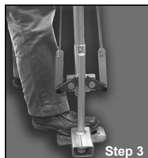
**Step 3:** Place unit so that jaws are on either side of stake adapter bar and continue as noted in Operating Instructions.
