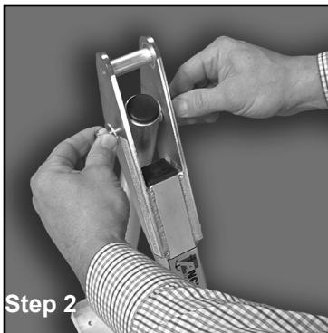
**Step 2:** Start 3/8" - 24 self-locking nut onto bolt.
