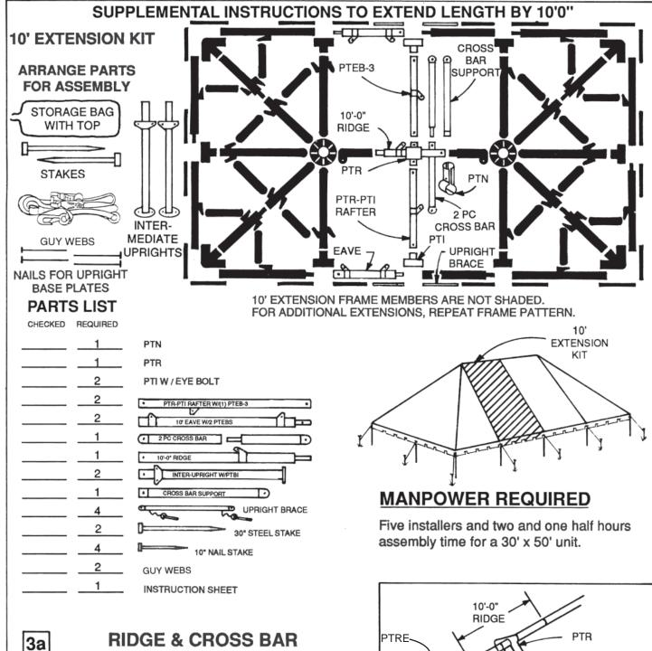
Slide PTR on to 10'-0" ridge. Align with hole at center of ridge and pin. Repeat for each 10'-0" ridge. Pin 10'-0" ridges together and add existing ridges to each end. Lift and pin assembled ridges to PTT's, using the PTRE pointed downward so that ridges are elevated.
