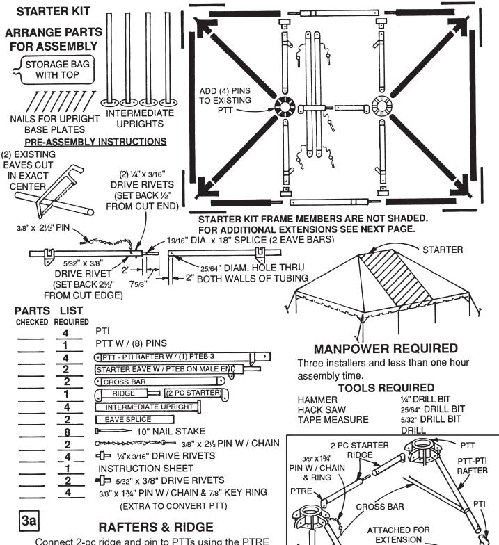
Connect 2-pc ridge and pin to PTTs using the PTRE pointed downward so that the ridge is elevated.
