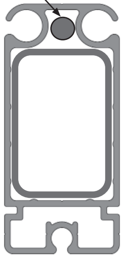
Cross sectional view of upright.
