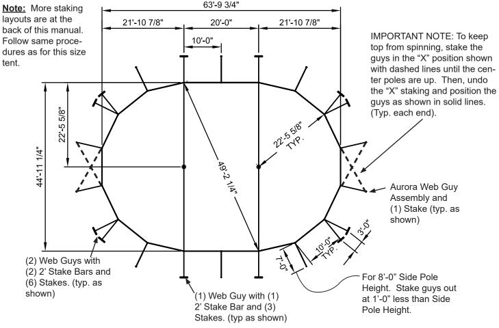
**Stake and Pole Layout for Tent:** Using the Installation Layout Cable and/or the staking layout appropriate for your size tent, mark placement of Center Poles, Side Poles and Stakes. See separate instructions for Installation Layout Cable use.
