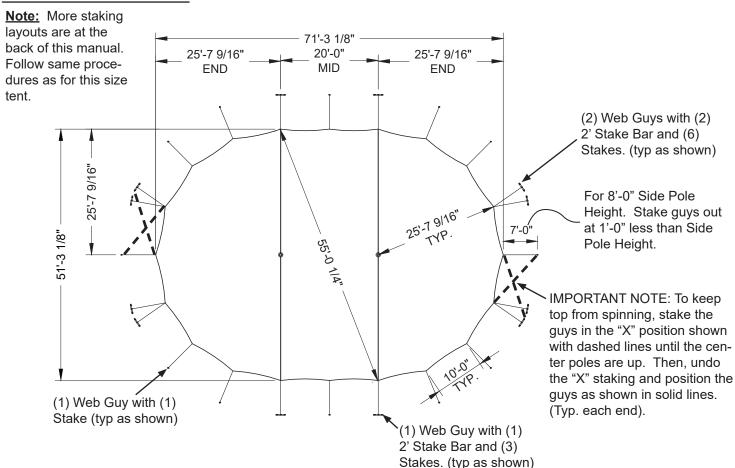
**Stake and Pole Layout for Tent:** Using the Installation Layout Cable and/or the staking layout appropriate for your size tent, mark placement of Center Poles, Side Poles and Stakes. See separate instructions for Installation Layout Cable use.
